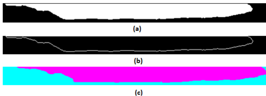
Figure 6. (a) binary image (b) perimeter of image (c) after image labelling ( J_G=0.51 m/s and J_L=0.77 m/s)
