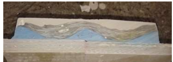
Gambar 23 Penampang potongan model sambungan tirus-dalam (TD-2)
