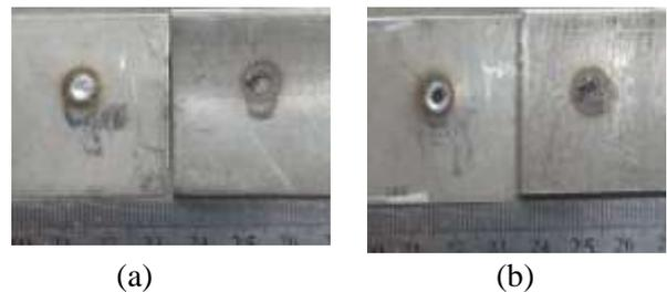
**Gambar 6** (a) Model Interfacial failure (IF),
