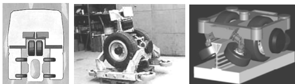
(a) Alweg (b) Steel box beam (c) Inverted T Gambar 2. Model footprint monorel jenis straddle (sumber: http://www.monorail.org )
