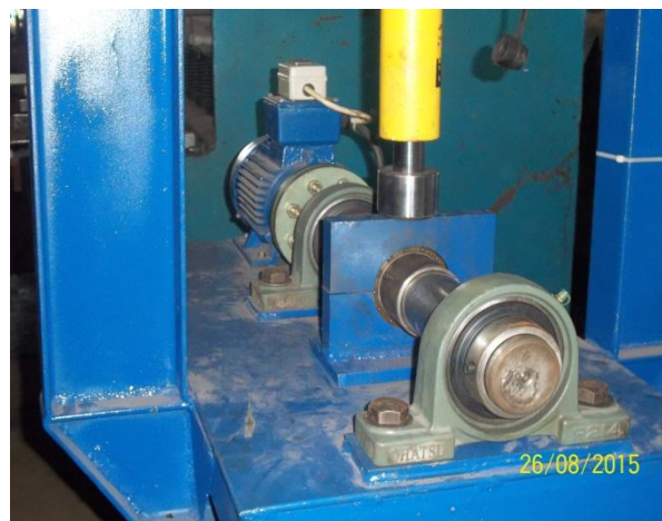
Gambar 3. Alat bantu kerusakan anti-friction bearing
