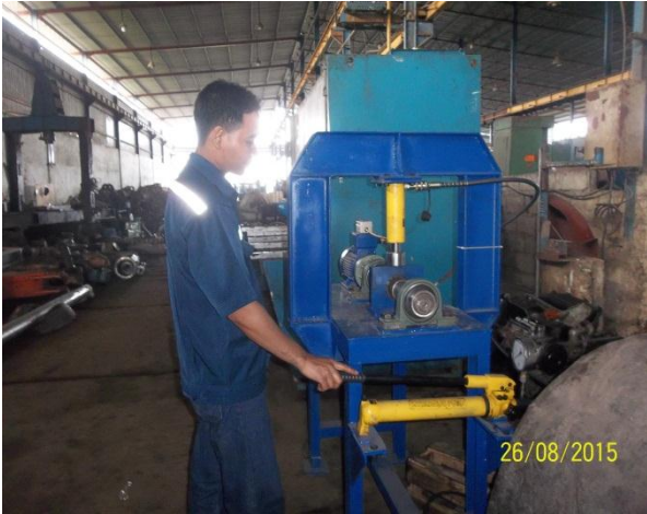
Gambar 4. Suasana uji coba alat bantu kerusakan anti-friction bearing
