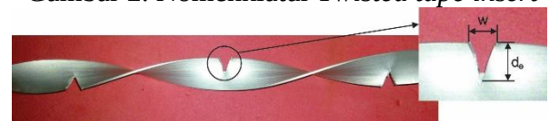
Gambar 3. Nomenklatur V-cut twisted tape insert
