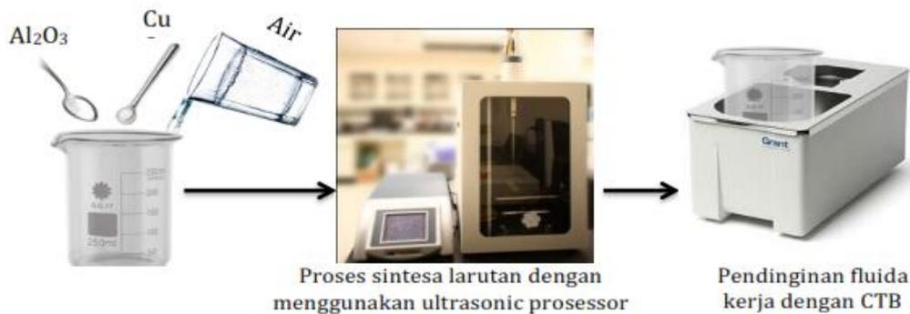
Gambar 2. Sintesa *hybrid nanofluid* Al<sub>2</sub>O<sub>3</sub>-CuO-Air.
