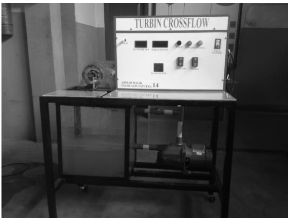
Gambar 3. Instalasi prototipe turbin Cross-flow
