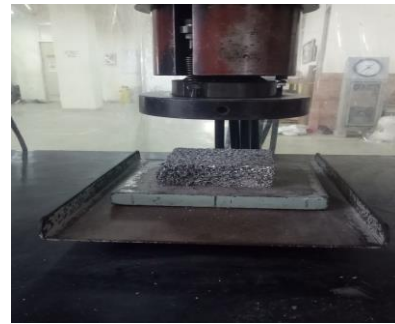
Gambar 5. Pengujian tekan aluminium foam
