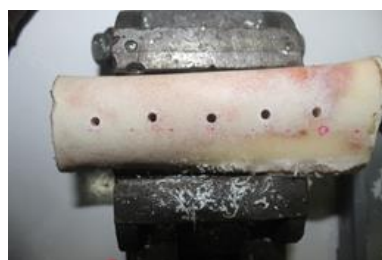
Gambar 4. Lubang hasil proses drilling
