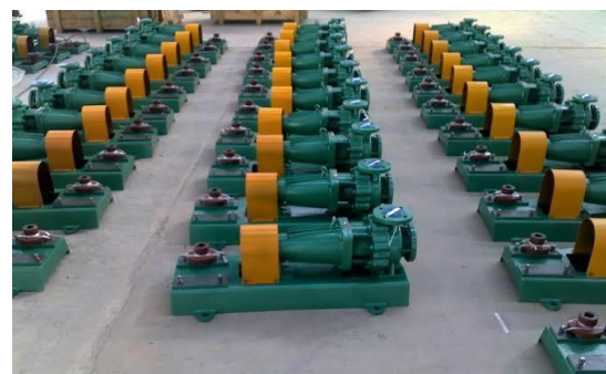
Gambar 4.6 pompa IHF fluorine plastic alloy single stage single suction kimia pompa sentrifugal.
