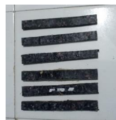
GAMBAR 3. Spesimen uji 3 point bending (ASTM D790 - 02)
