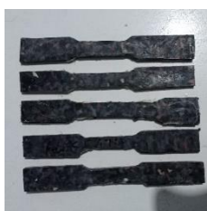
GAMBAR 2. Spesimen uji tarik (ASTM D638-3)
