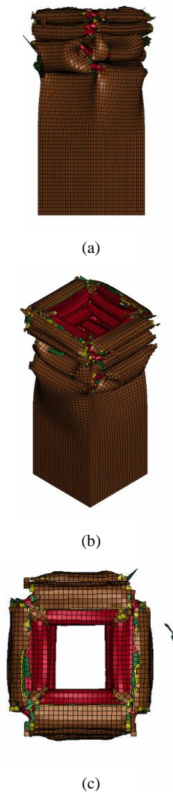
Gambar 7. Hasil simulaasi numerik hibrid aluminum/GFRP 3 lapisan komposit (a) front view (b) side view , (c) top view
