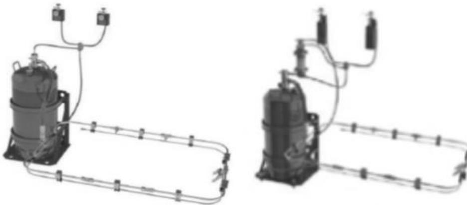
Gambar 1. Automatic fire suppression system
