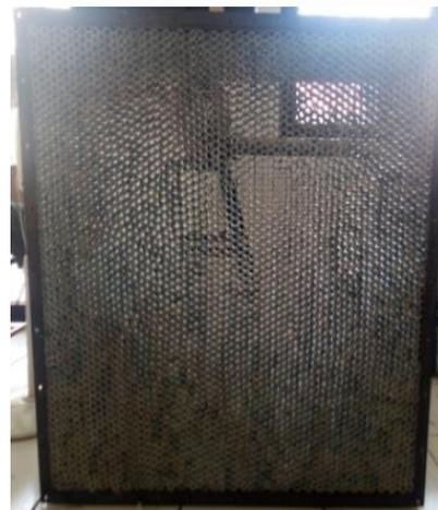
Gambar 3. Penampang flow straightener
