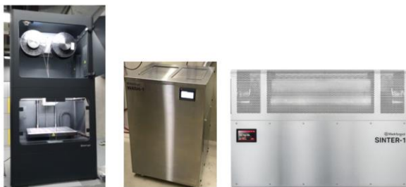
Figure 3 Markforged Metal X, Markforged Wash-1 dan Markforged Sinter-1 (from left to right)
