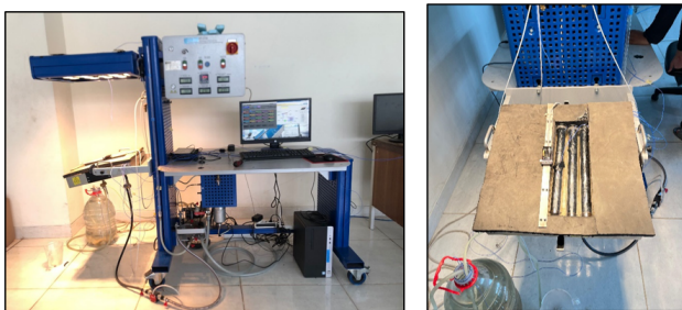
Gambar 2. Alat uji Principle of Solar Thermal Energy ET 202.
