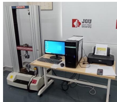
Gambar 2. Mesin uji tarik model HT-24-02
